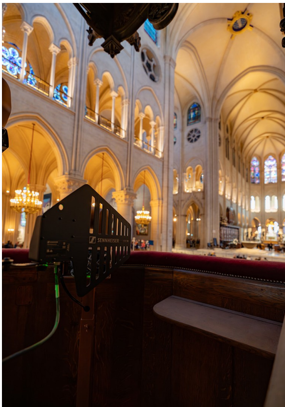
Unlike traditional RF wireless systems, Spectera does not employ diversity, which halved the antenna requirement for Notre-Dame (Photo credit: Olivier Allard)
